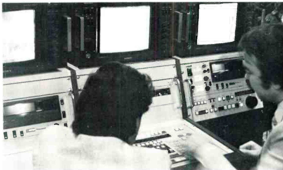
Demonstration of Sony's new editing system showing complete interfascibility of BVU-800 deck (right) with new Betacam 1/2-inch player (left)
