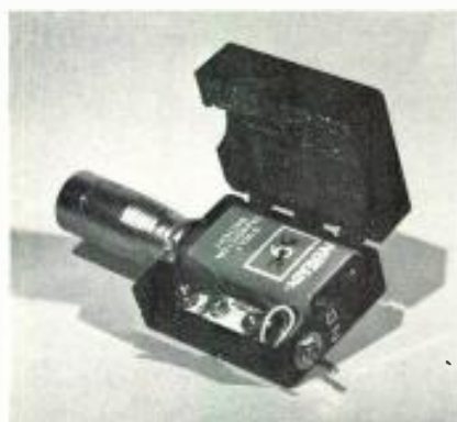
Audio signal generator diagrammed on previous page is depicted at left and below in completed form
