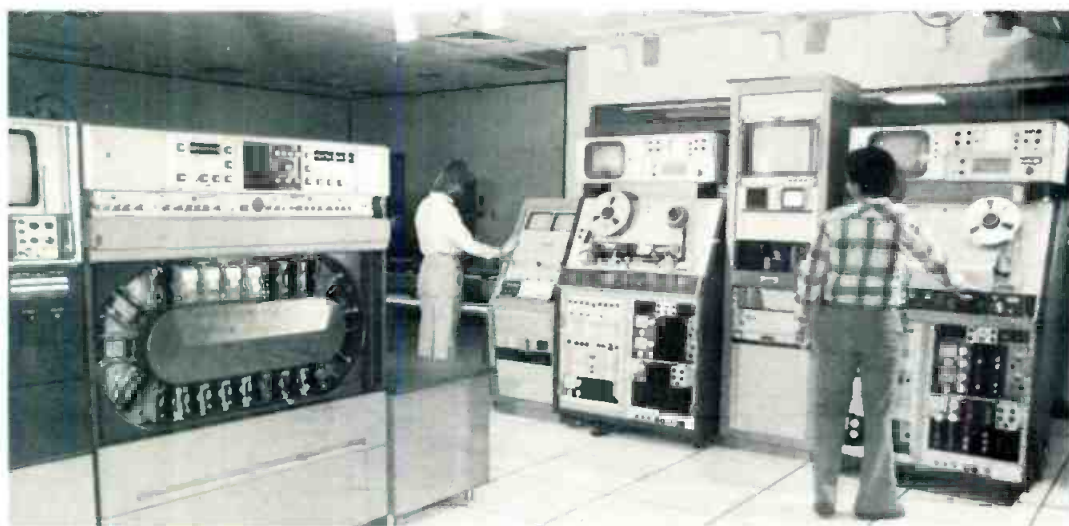
The videotape area at KBAK-TV features an RCA TCR-100 cart machine, Ampex VR-1200 quad machines, and Panasonic NV-9600 recorders
